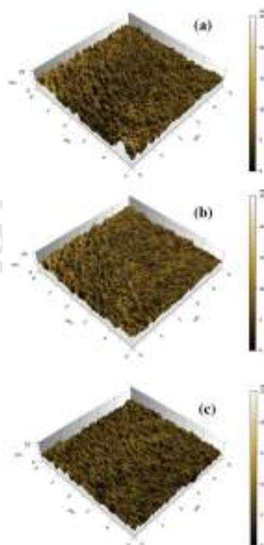
**Fig. 7** AFM height images of the films made from the photoactive blend of PBDB-T:Cu<sub>2</sub>S:ITIC with (a) 0 wt % Cu<sub>2</sub>S NCs, (b) 6 wt % Cu<sub>2</sub>S NCs and (c) 8 wt % Cu<sub>2</sub>S NCs.
