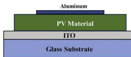
Fig. 1. Side face of fabricated PV cell.
